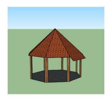
The kiosk was containing the water pump that was used to bring up water into the water tower. It was activated by a donkey. It is 4.5m high, and 10m diameter.
